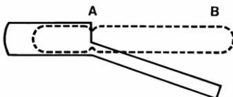
Side view of ampoule opening device containing an ampoule positioned ready to open. 'A' is the score mark and 'B' the point of applied pressure.
